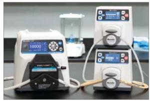
The L/S digital Miniflex pump system (aboove right) requires less than half the bench space when compared to the L/S standard digital drive (above left).
